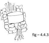
Suitable for preparing food for many number of persons. Any type of food can be prepared. Can be made using bricks or stones. Having ability to construct according to the size of the container is an advantage. Ability to make easily is also a special advantage.
